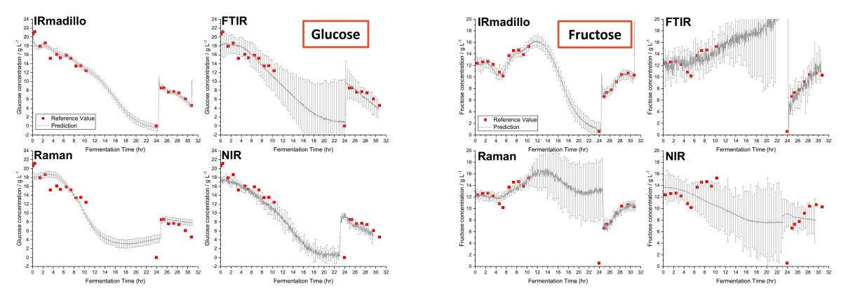
All four instruments track general consumption of glucose. Uncertainty on FTIR is very large, and Raman struggles to predict absolute concentrations, especially at end stage of fermentation. Neither Raman nor NIR measure the "0" value of glucose.
