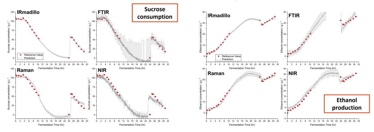
All four instruments are capable of measuring both sucrose consumption and ethanol production over the course of the fermentation. All of the spectrometers show the step change caused by the sucrose addition at 25 hr, but only the IRmadillo and FTIR accurately model the new sucrose concentration afterwards. FTIR measures unrealistically high values for ethanol.
